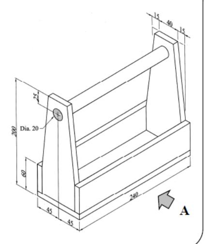
The diagram shows a pictorial drawing of a small display shelf. All material is 15mm thick.
