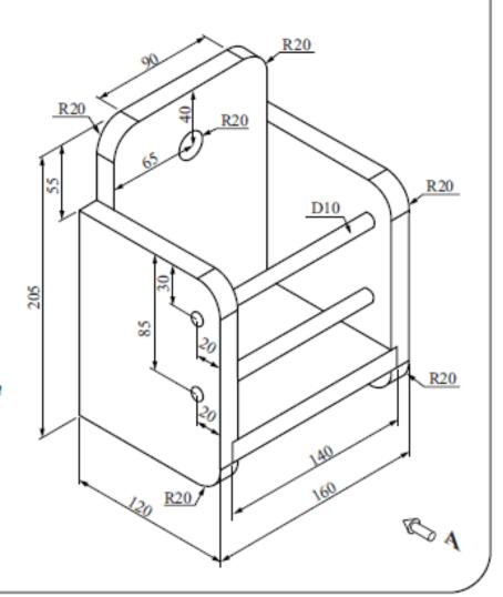
2. The diagram shows a pictorial drawing of a bookend. All material is 20mm thick.
