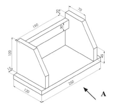
The diagram shows a pictorial drawing of a small toast rack. All material is 15mm thick.
