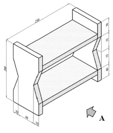
The diagram shows a dimensioned isometric drawing of a bookshelf.
