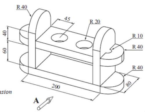
The diagram shows an isometric drawing of a storage rack.
