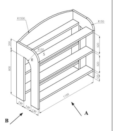
(ii) With the aid of notes and neat freehand sketches, describe a suitable method of joining the members R and S.
